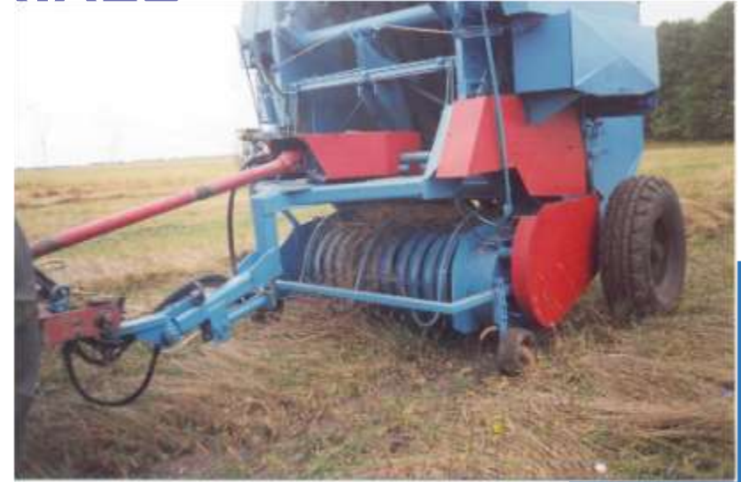
Photo of a universal round baler with a pickup and an improved bale chamber
